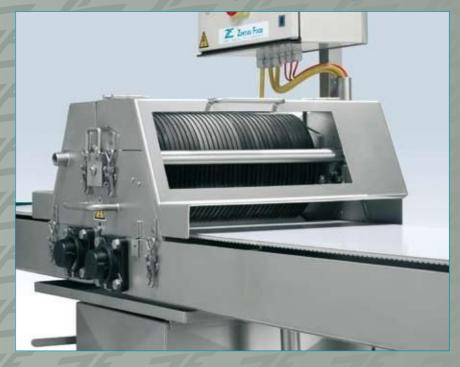
The removable knife unit has been mounted in a tipping system which is guarded by a removable cover. The special frame construction and quick release system ensure that the conveyor belts can be fully removed, both easily and quickly.
